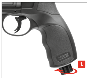
1. Unscrew the retaining screw.
